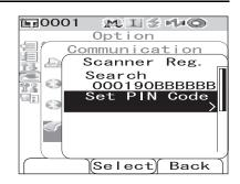
$\label{eq:constraint} 2 \quad Use the \lhd or \triangleright button of the cross key to move the cursor, and use the \triangle or \bigtriangledown button to change the value.$
