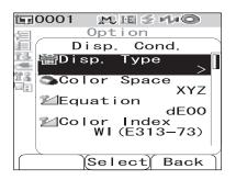
**3** After you set the display conditions, press the [TARGET] (Back) button to return to the <Option> screen.
