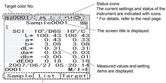
The functions assigned to the [SAMPLE], [SAVE/SEL] and [TARGET] buttons are displayed respectively.
